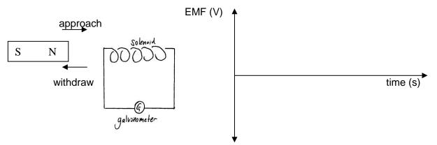
Indicate current direction in the solenoid circuit as the magnet approaches. Put an arrow on the diagram and label it current.
