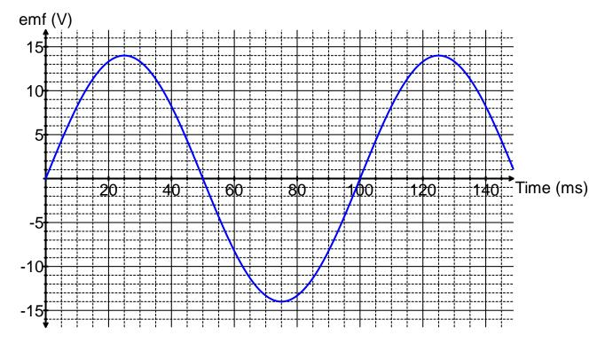
f) Determine the RMS voltage of this AC generator
